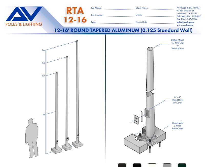
**SHAFT:** One-piece extruded 6063 aluminum alloy tube heat treated to a T6 temper. Shaft has a uniform taper.
