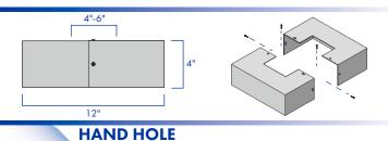
HAND HOLE: Reinforced 3" × 5" hand hole is located 18" above base. Cover and attachment hardware provided.
