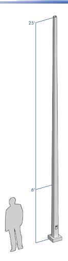
**SHAFT:** Commercial-quality, hot-rolled, carbon steel tubing with a minimum yield strength of 55,000 PSI, conforms to ASTM A595 grade A. Shaft has a uniform taper of 0.14" per foot.
