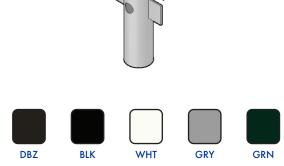
**FINISH:** TGIC thermoset polyester powder coat finish is electrostatically applied at a 3.0 mil minimum thickness. A five stage metal pretreatment process and sealer provide maximum corrosion resistance. The powder top coat is baked in excess of 400 degrees for supreme endurance.
