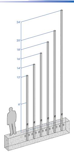
**SHAFT:** Commercial-quality, hot-rolled, carbon steel tubing with a minimum yield strength of 46,000 PSI, conforms to ASTM A500 grade B.
