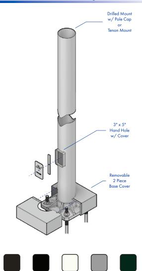
**FINISH:** TGIC thermoset polyester powder coat finish is electrostatically applied at a 3.0 mil minimum thickness. A five stage metal pretreatment process and sealer provide maximum corrosion resistance. The powder top coat is baked in excess of 400 degrees for supreme endurance.
