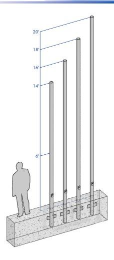
**SHAFT:** Commercial-quality, hot-rolled, carbon steel tubing with a minimum yield strength of 46,000 PSI, conforms to ASTM A500 grade B.
