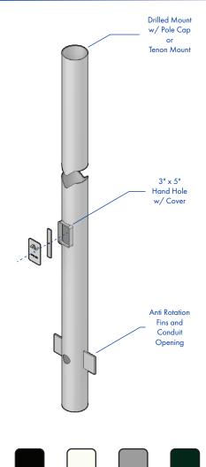
**FINISH:** TGIC thermoset polyester powder coat finish is electrostatically applied at a 3.0 mil minimum thickness. A five stage metal pretreatment process and sealer provide maximum corrosion resistance. The powder top coat is baked in excess of 400 degrees for supreme endurance.
