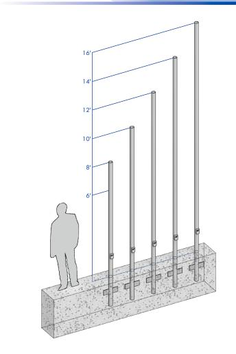
**SHAFT:** Commercial-quality, hot-rolled, carbon steel tubing with a minimum yield strength of 46,000 PSI, conforms to ASTM A500 grade B.
