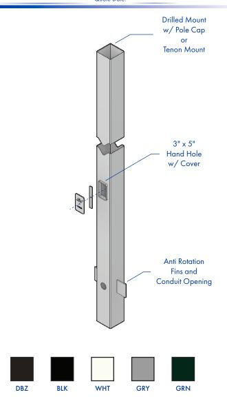
FINISH: TGIC thermoset polyester powder coat finish is electrostatically applied at a 3.0 mil minimum thickness. A five stage metal pretreatment process and sealer provide maximum corrosion resistance. The powder top coat is baked in excess of 400 degrees for supreme endurance
