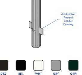
**FINISH:** TGIC thermoset polyester powder coat finish is electrostatically applied at a 3.0 mil minimum thickness. A five stage metal pretreatment process and sealer provide maximum corrosion resistance. The powder top coat is baked in excess of 400 degrees for supreme endurance.
