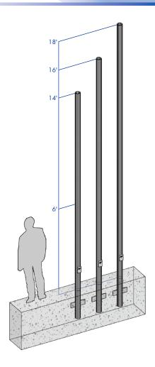
**SHAFT:** One-piece extruded 6063 aluminum alloy tube heat treated to a T6 temper.
