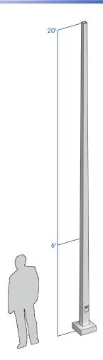
**SHAFT:** Commercial-quality, hot-rolled, carbon steel tubing with a minimum yield strength of 55,000 PSI, conforms to ASTM A595 grade A. Shaft has a uniform taper of 0.14" per foot.
