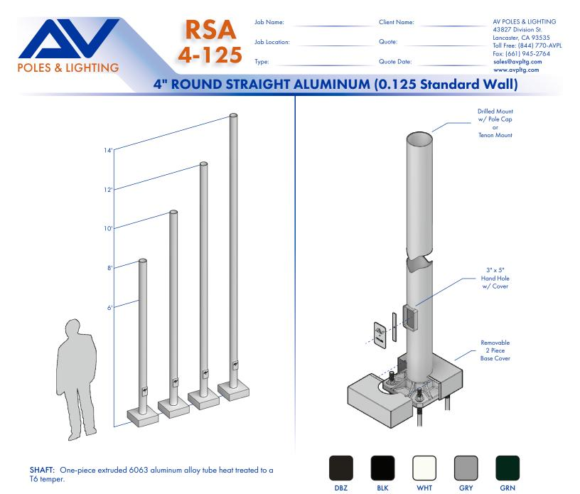
**GROUNDING:** Provision; 3/8-16 Threaded stud welded to inner shaft wall opposite hand hole. Flat washer and hex nut provided.
