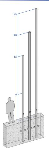
**SHAFT:** Commercial-quality, hot-rolled, carbon steel tubing with a minimum yield strength of 46,000 PSI, conforms to ASTM A500 grade B.
