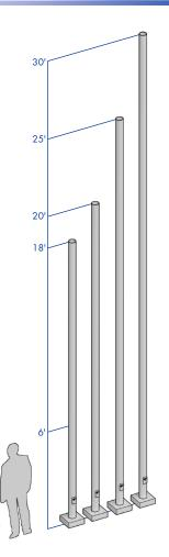
**SHAFT:** Commercial-quality, hot-rolled, carbon steel tubing with a minimum yield strength of 46,000 PSI, conforms to ASTM A500 grade B.
