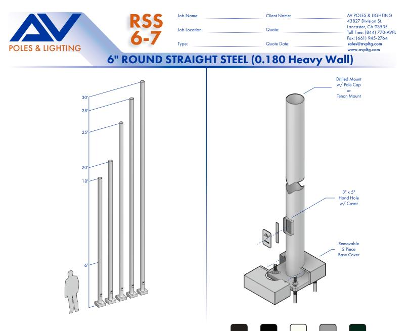
**SHAFT:** Commercial-quality, hot-rolled, carbon steel tubing with a minimum yield strength of 46,000 PSI, conforms to ASTM A500 grade B.
