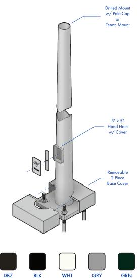
**FINISH:** TGIC thermoset polyester powder coat finish is electrostatically applied at a 3.0 mil minimum thickness. A five stage metal pretreatment process and sealer provide maximum corrosion resistance. The powder top coat is baked in excess of 400 degrees for supreme endurance.
