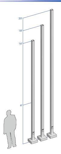
SHAFT: One-piece extruded 6063 aluminum alloy tube heat treated to a T6 temper.
