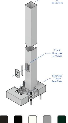
**FINISH:** TGIC thermoset polyester powder coat finish is electrostatically applied at a 3.0 mil minimum thickness. A five stage metal pretreatment process and sealer provide maximum corrosion resistance. The powder top coat is baked in excess of 400 degrees for supreme endurance.
