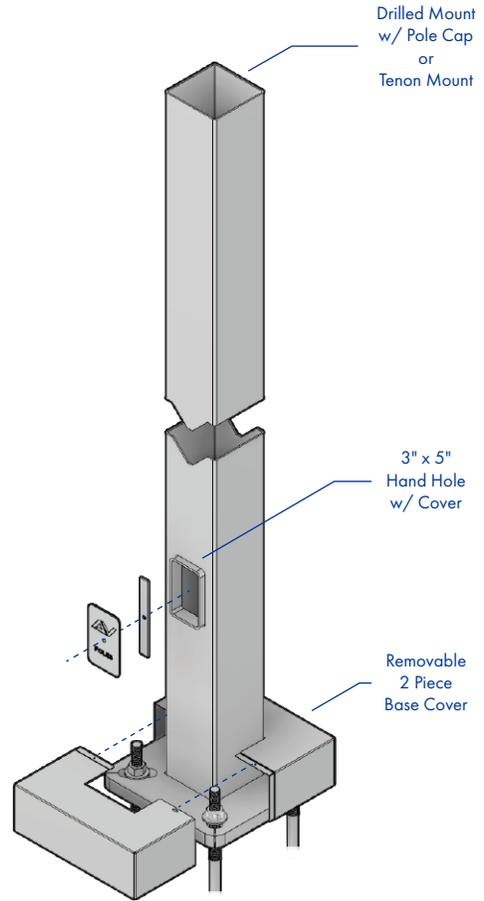
**SHAFT:** Commercial-quality, hot-rolled, carbon steel tubing with a minimum yield strength of 48,000 PSI, conforms to ASTM A500 grade A.
